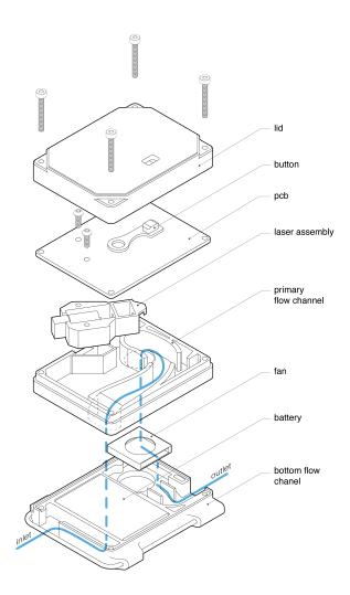
Figure 5. An exploded drawing of the MyPart Design detailing the airflow and laser placement.
