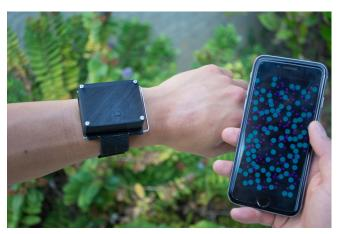
Figure 1. The small wrist-worn MyPart sensor and optional accompanying smartphone visualization and data logging app.
