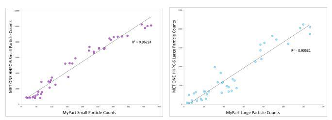
Figure 7. Graphs demonstrating the performance of MyPart (\$50 US) in correlation with the calibrated Met-One HHPC6 (\$4000 US).
