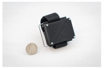
Figure 4. MyPart configured as a wrist worn device (40x55x23mm) with LED particle count display illumniated.
